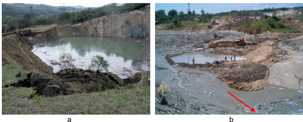
Fig. 1. The evolution of the local pollution phenomenon in the Ocnele Mari extraction area: a – view of the cavern after the implosion (year 2001); b – local pollution of the land through the discharge of brine (year 2004) [Luca and Tigaret 2008].
